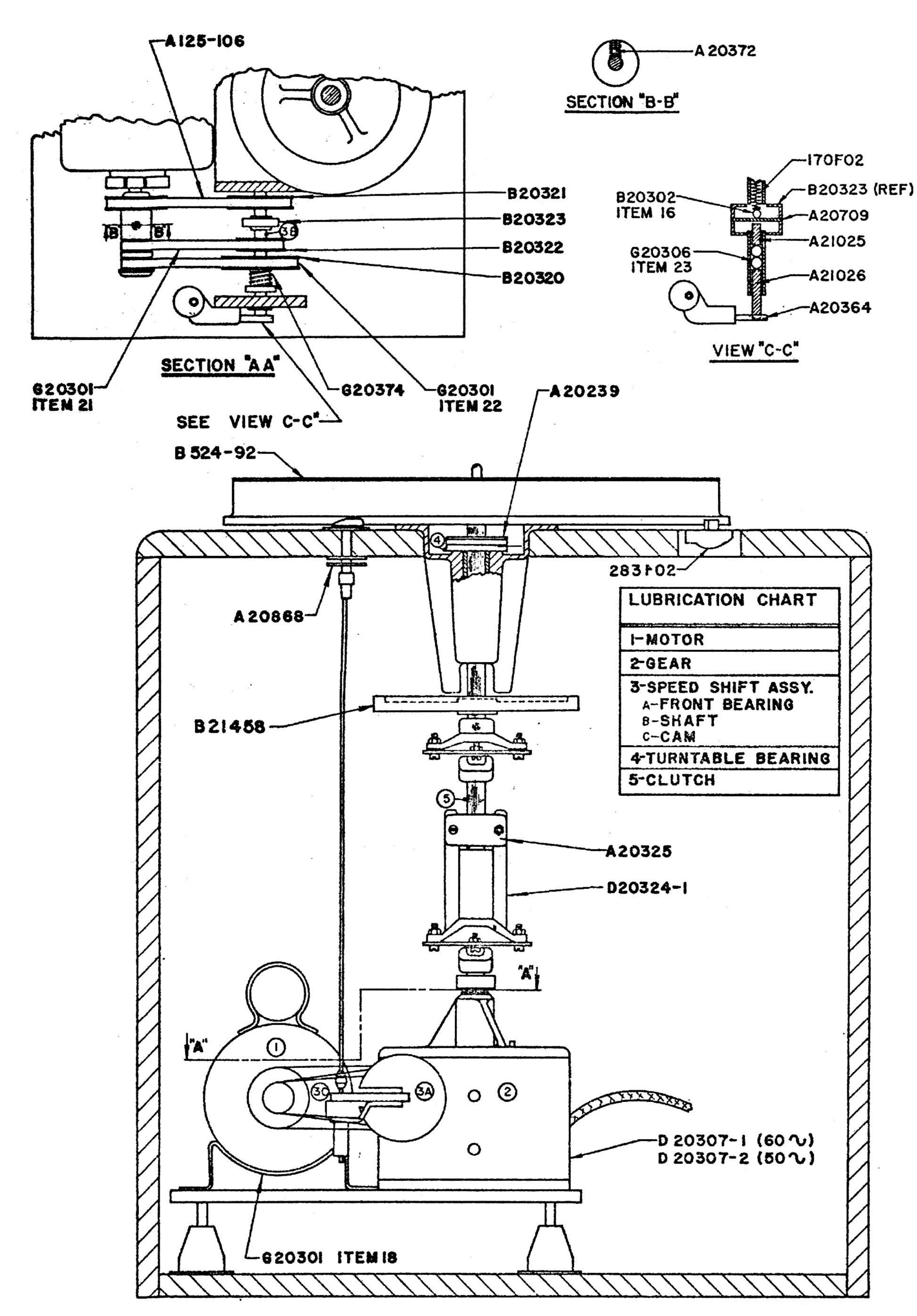
REPLACEMENT PARTS AND LUBRICATION CHART FIG. I
